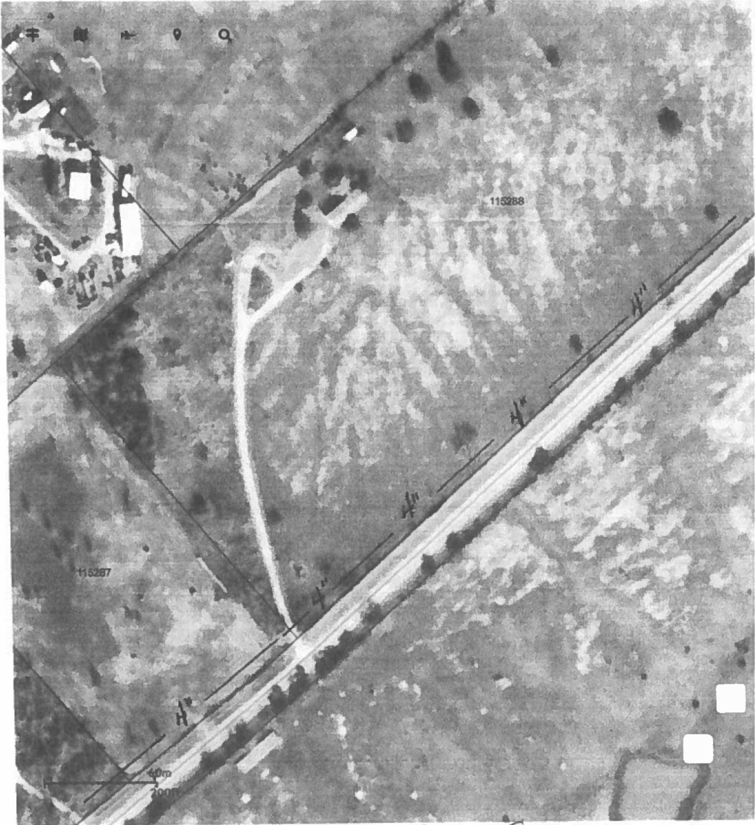
4" PVC ACROSS entire front of property ALONG FM 2D
